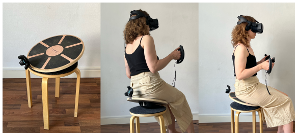
Figure 6: The VR implementation using a custom balance board interface, where users navigate by leaning toward their desired direction.
