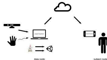
The second data cycle concerns the horizontal updates between concurrent nodes running the application. In this scheme, while each device running the application controls locally its own avatar, it also hosts passive instances of the avatars controlled by remote nodes. Each local instance, besides performing the data cycle described before, is responsible for uploading its state changes to the cloud, at regular intervals, so as to inform its instances hosted on remote nodes. (Figure 4).
